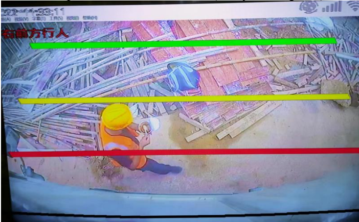
Front right BSD camera diagram
