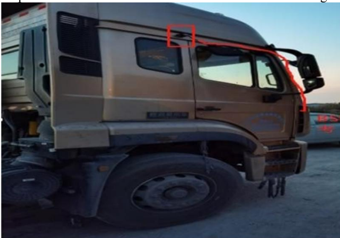
Front right BSD camera diagram
