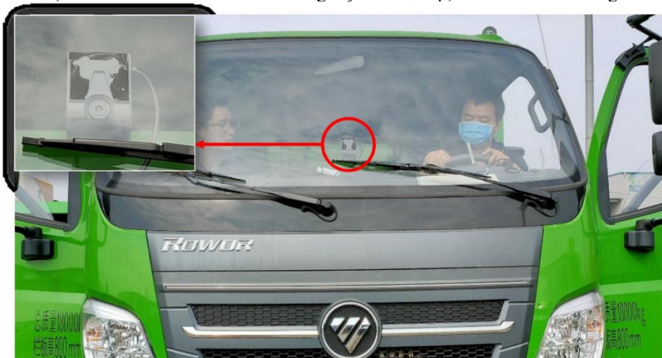
Effect picture of ADAS pre installation
